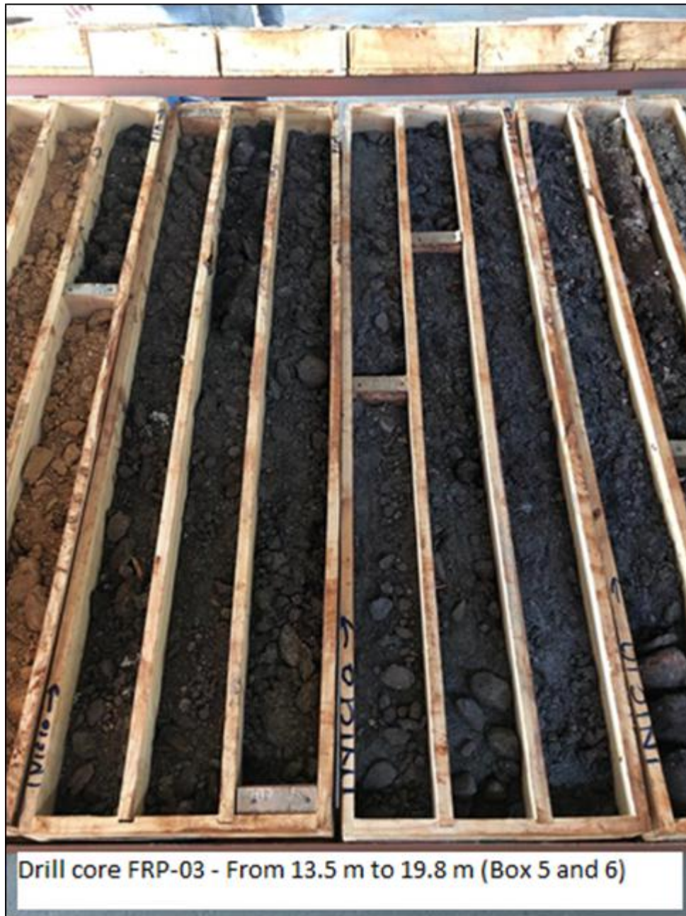
Figure 6.3.2-1: Friable Siliceous Itabirite. Drill core: FRP 03.
